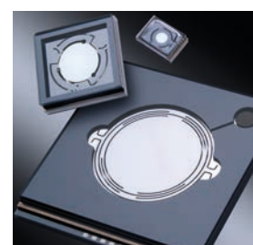
MEMS mirrors with diameters of 2 mm up to 20 mm.
